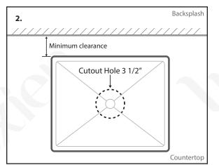
2. Once the placement has been determined. Mark the center of the drain hole and set aside the vessel sink. Draw a 3 1/2 inch diameter circle around the center of the drain hole. Use a jigsaw or a power tool to cut the opening on the mounting surface.
