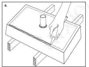
4. Place the assembled vessel sink through the 3 1/2" opening on the counter top and check for level and fit. Plumber's putty can be used to level the sink. Apply silicon adhesive around the bottom rim of the sink as shown.
