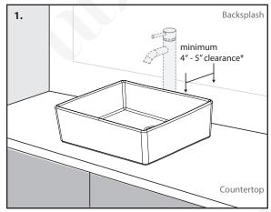
1. It is highly recommended to have all the necessary parts on the job site to determine the optimal placement prior to installation. (**\*NOTE:** Minimum clearance distance is required for vessel sinks without a faucet mounting hole)
