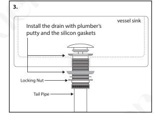
3. Attach the pop up drain to the ceramic sink as shown. It is recommended to use plumber's putty with the silicon gaskets to prevent any possible water leak. Make sure the drain is properly secured to the vessel sink.
